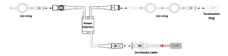
By using ENTTEC's Smart PXL Power Injector 24v accessory (SKU: 73019) to inject power from additional PSU's, the impact of voltage drop and power consumption can be removed leaving control channel availability as the only limiting factor.
