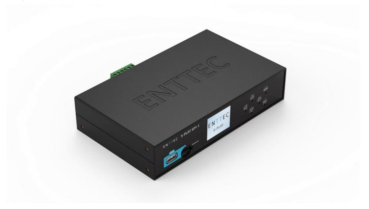
ENTTEC's S-PLAY is a highly accurate, 32 universes show controller and lighting record / playback device.
