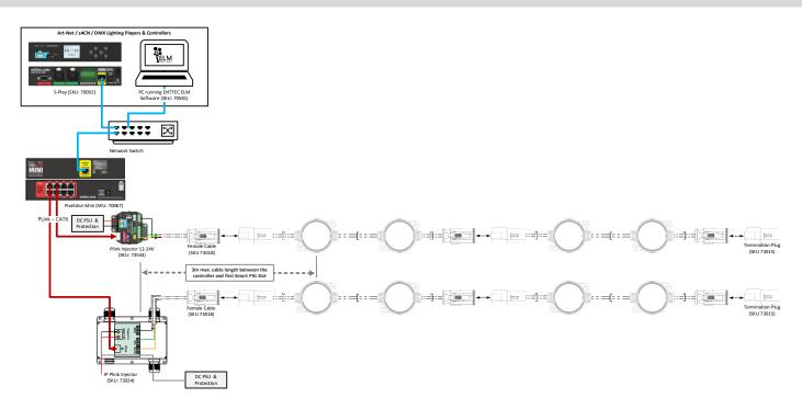
Note: If the power or data source to your controller drops out whilst the Smart PXL Dots remain powered, the last state will be held until either the data feed resumes or power to the Smart PXL Dots is disconnected and reconnected.
