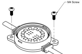
Position each Smart PXL Dot in-line with the entry points, then insert and fully tighten the screws. **DO NOT** exert any tension on the cabling whilst tightening.
