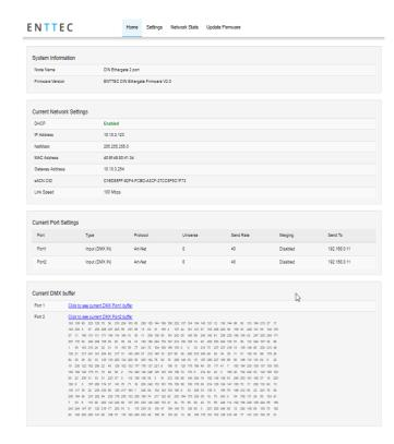
Current DMX Buffer: The Current DMX buffer displays a snapshot of all current DMX values when refreshed manually.
