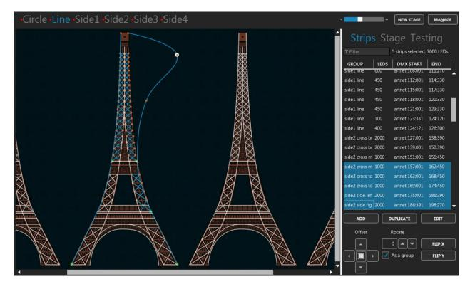
You can create as many stages as you want. Generally, you'll want an overall stage corresponding to the whole installation and multiple individual stages to target specific zones. The overall stage allows you to map content across the board. Then the other stages allow you to override specific parts of your installation whenever you want. You can select the current stage by clicking its name at the top.
