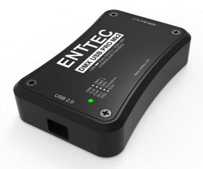
The DMX USB PRO MK2 can control up to 1024 DMX channels or receive them through one simple USB 2.0 connection. Compatible with a broad array of supported 3rd party commercial and free software running on Windows, Linux or MacOS.
