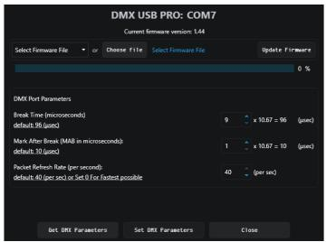
From EMU interface, click on "Select Firmware file" to select from drop down list for default firmware option, or download FW from ENTTEC website and locate it manually with "Choose File". Firmware 2.4 is needed, if DMX USB PRO is to be used with RDM Controller Application
