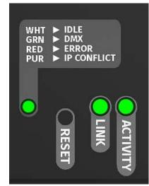
LINK: is ON when there is an active Ethernet Link @ 100 mbps. It will stay OFF @ 10 mbps.
